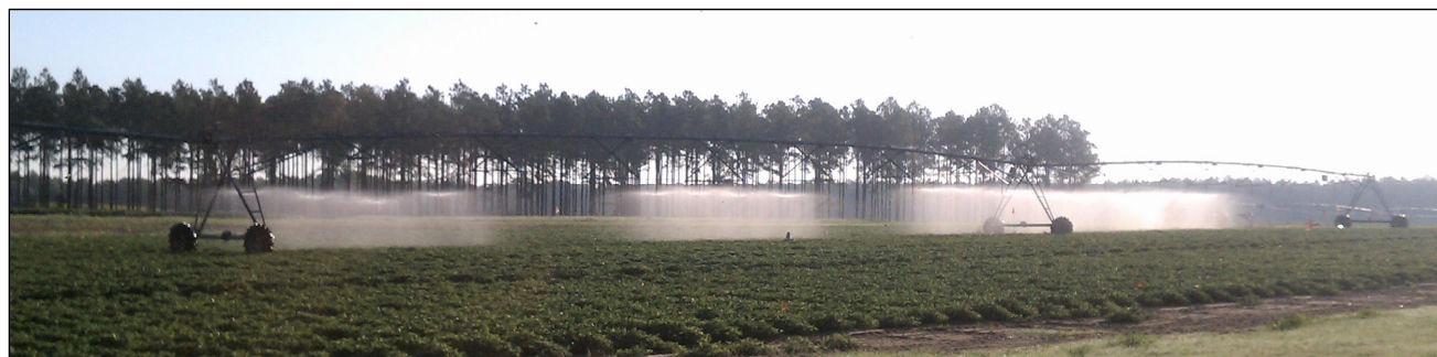
Figure 6. Variable rate irrigation enabled pivot at the University of Georgia’s Stripling Irrigation Research Park applying different irrigation rates over research plots.
